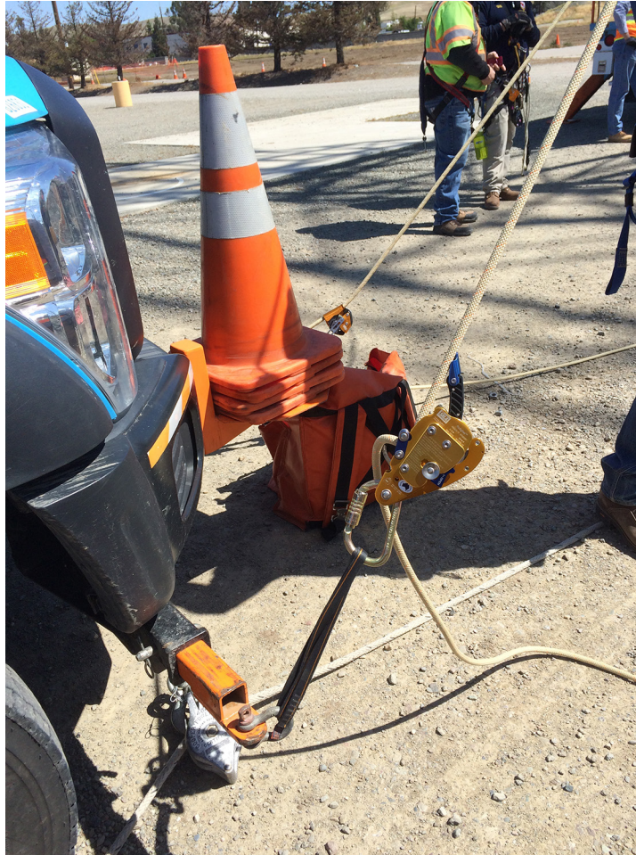
Figure 4.1.B.1. Ground-Based Anchor Point.
