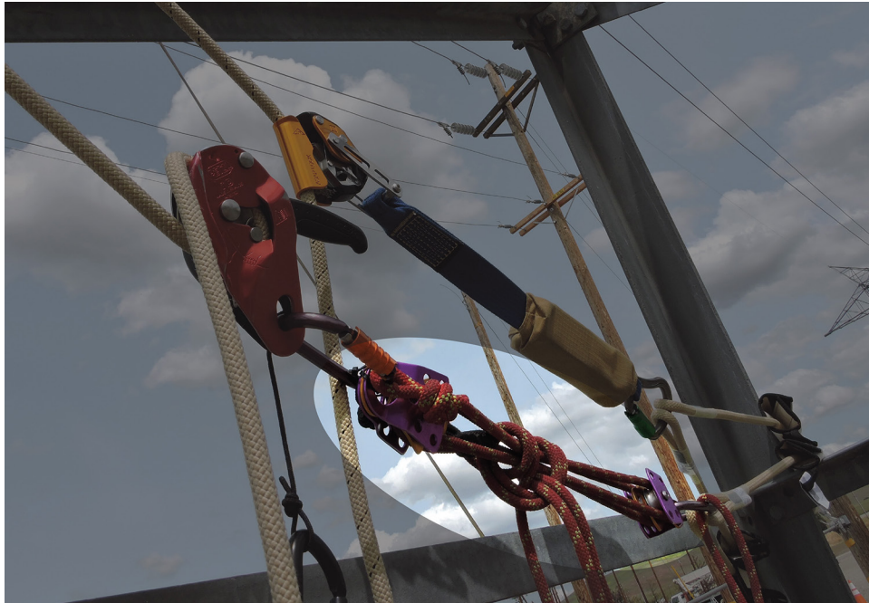
Figure 4.2.2. Ropes Tied Off With Two Half Hitches.
