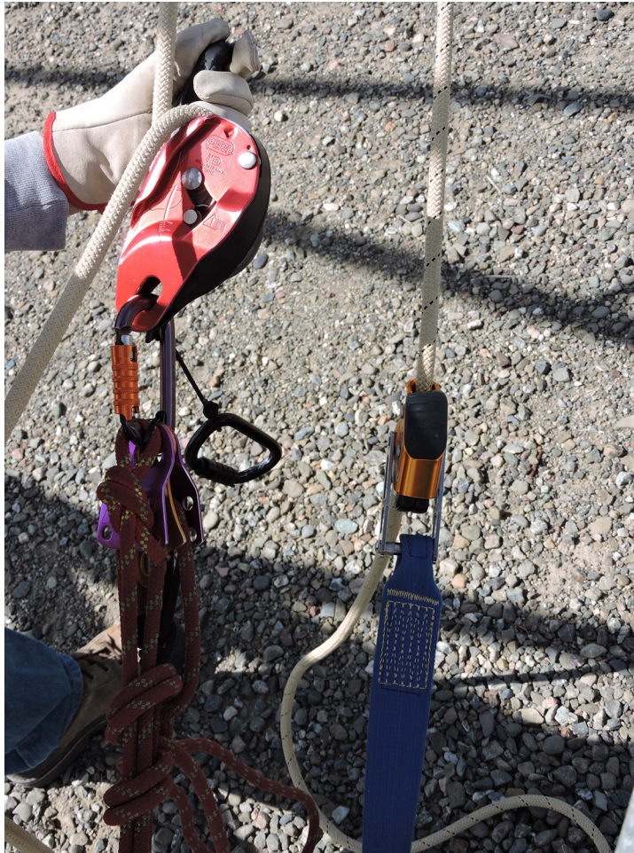
Figure 4.1.B.5. Controlling the Primary and Secondary Decent Devices
