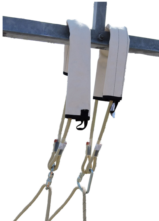
Figure 4.1.A. Provide Adequate Distance Between Anchor Straps.
