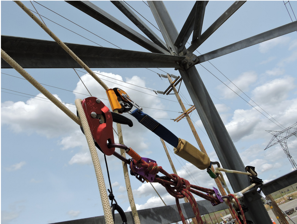
Figure 4.2.1. View of a Descender and Secondary Device Connected in a Structure.
