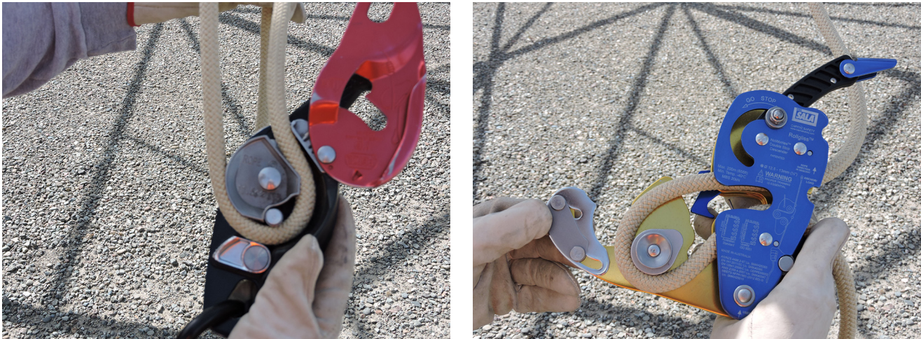
Figure 4.1.B.2. Connecting the Primary Rope to the Descender
